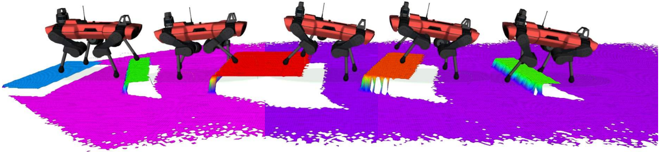
Fig. 5. Snapshots of a Gazebo simulation where the ANYmal C robot walks over obstacles of 6, 12 and 18 cm while replanning its base pose, its linear and angular velocity and contact locations at 1.5 Hz adapting to the latest height map using the TO formulation presented in Sec. IV-B.
