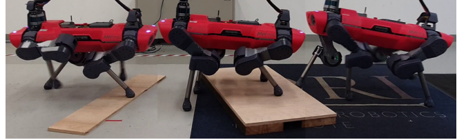
Fig. 10. The initial guesses provided by the LMTR trained on flat-ground can be adapted to mild height variation of 0.02 m to 0.08 m by the receding-horizon optimization, showing the ability to cope with minor imprecisions.
