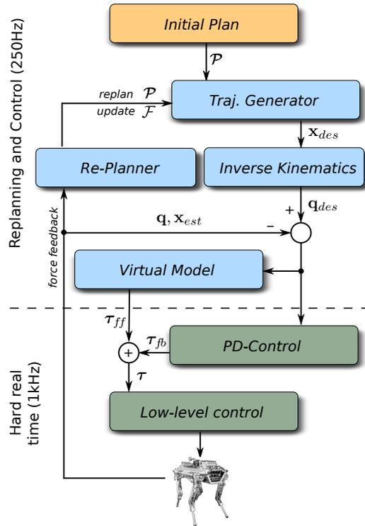
Fig. 1. Control loop to robustly execute a motion plan  $P$ . The desired states are mapped to joint angles using inverse kinematics. From these desired joint states feed-back and feed-forward torques are calculated to create the compliant behaviour. In a feedback-loop the joint torques are used to estimate the contact forces at the feet and update motion-plans accordingly.
