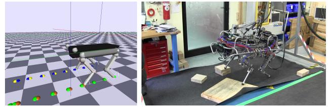
Fig. 3. *Left*: The internal map and motion plan of the robot. The task is straight walking on obstacle free terrain. *Right*: The robot successfully executing the planned motion despite unseen, randomly placed obstacles of up to 15cm height (20% of the leg length). The robot uses active compliance combined with force-based motion replanning.
