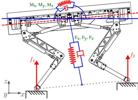
Fig. 2. The virtual elements used to calculate forces and moments around the trunk of the robot. The virtual forces and moments are transformed to forces at the feet and subsequently to feedforward torques for the legs that are in stance [7].
