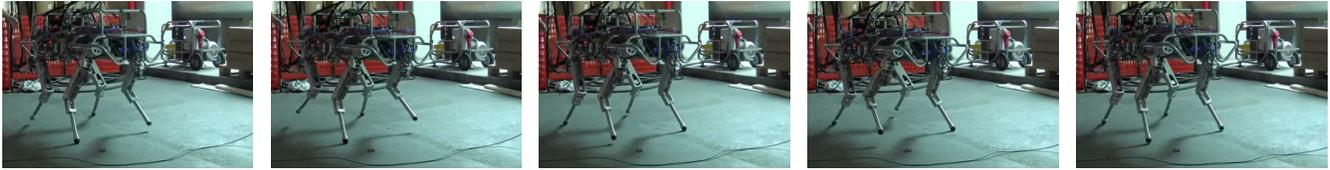
Fig. 10. Snapshots of a video of the HyQ robot trotting in place. From left to right: the swing legs are shortening while the support legs are supporting the robot's weight and correcting the posture. Two snapshots later the swing pair lands, the leg pairs switch and the state machine cycle continues. In the background the off-board oil pump that has been used throughout our experiments is visible. Link to video available at the Appendix.
