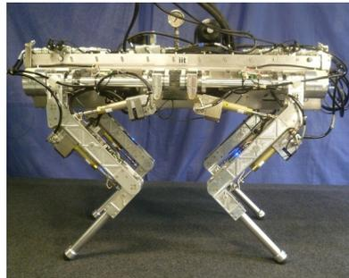
Fig. 1. The hydraulically actuated quadruped robot - HyQ. It has 12 degrees of freedom and its size is comparable to a goat. HyQ is designed for highly dynamic behaviour, e.g. trotting and jumping.
