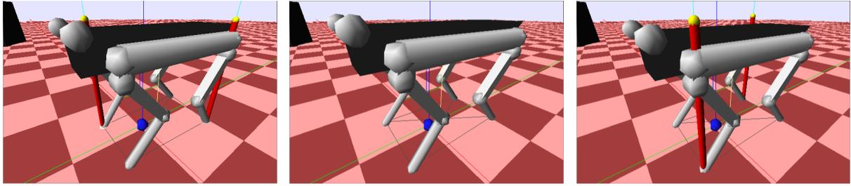
Fig. 2. HyQ trotting in place in simulation. The left and right images show the robot in two consecutive mid-stance phases. The middle image shows the robot in flight phase. The red cylinders represent ground reaction forces.
